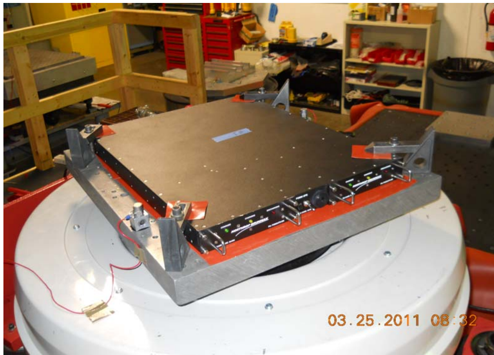
Figure 3-1: Test setup for vertical-axis composite wheeled vehicle vibration.
