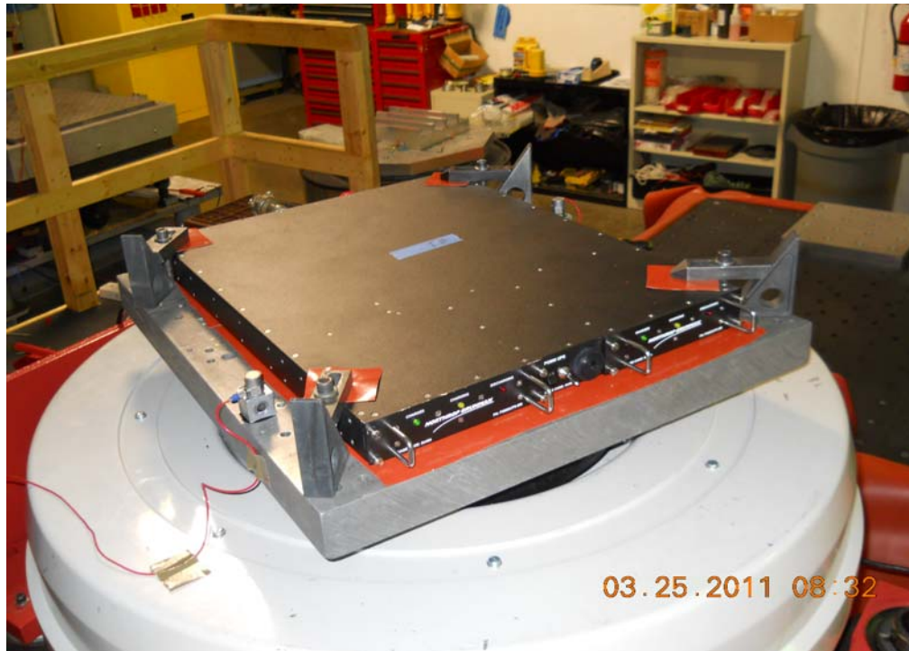
Figure 4-1: Test setup for vertical-axis SRS shock.
