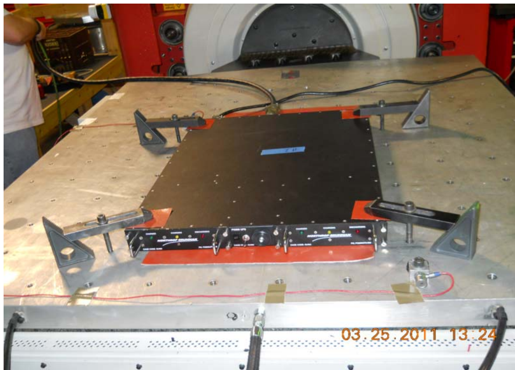
Figure 4-2: Test setup for longitudinal-axis SRS shock.
