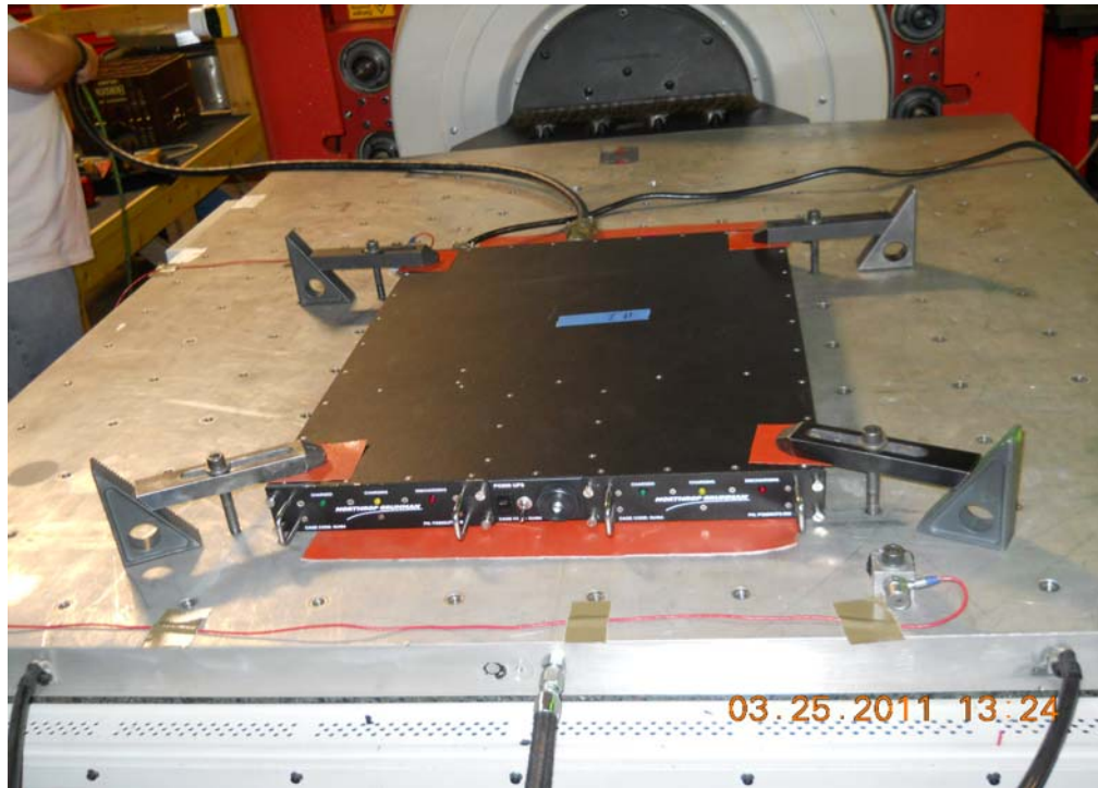
Figure 3-2: Test setup for longitudinal-axis composite wheeled vehicle vibration.
