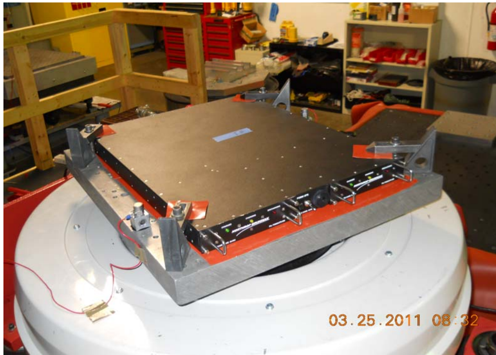
Figure 2-1: Test setup for vertical-axis SRS shock.
