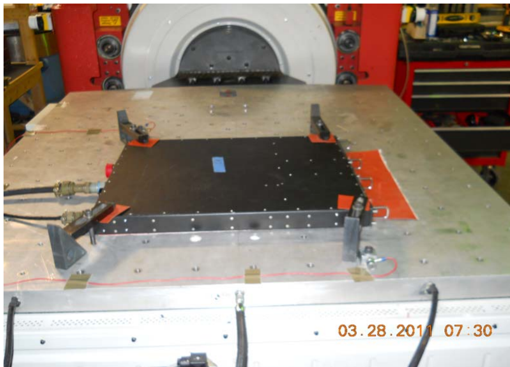
Figure 3-3: Test setup for transverse-axis composite wheeled vehicle vibration.
