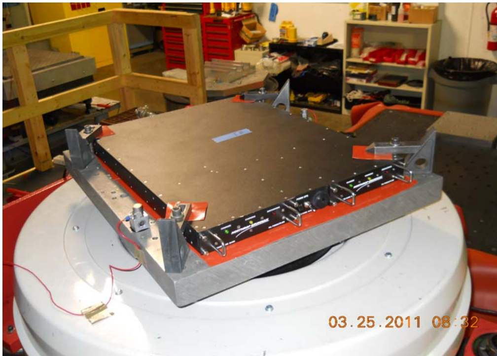
Figure 1-1: Test setup for vertical-axis composite wheeled vehicle vibration.
