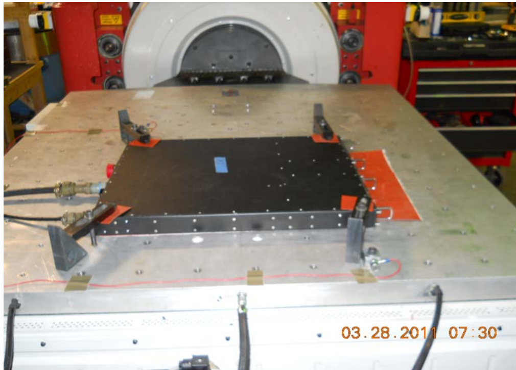
Figure 4-3: Test setup for transverse-axis SRS shock.
